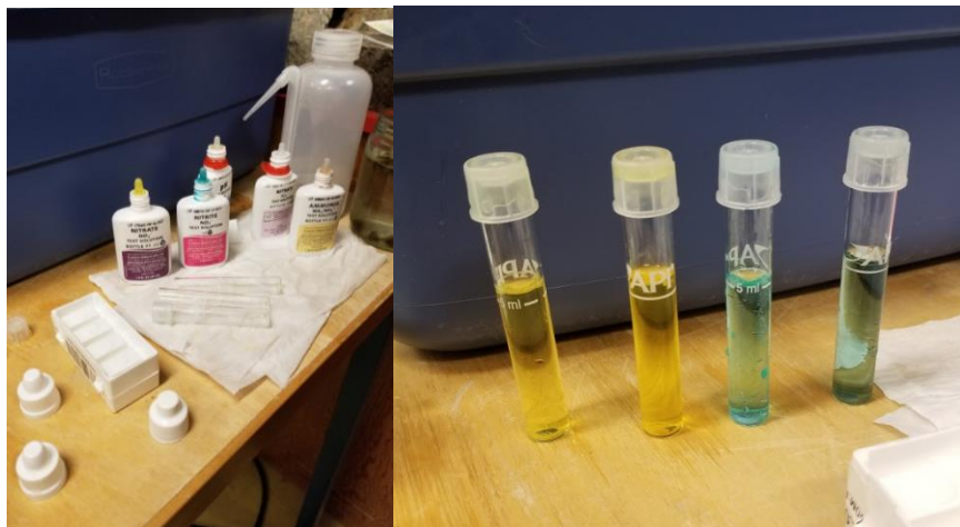
Figure 7: API Freshwater Master Kit used to test nutrient levels
