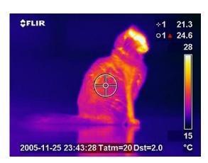
Figure 8. The true temperature of a target can only be estimated using a thermal camera if its emissivity coefficient is known. Image: FLIR.<sup>8</sup>
