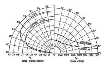
Figure 5. The effect of the angle of incidence on the perceived emissivity of various materials. Note how, when viewed between 80 and 90°, the emissivity of glass is lower than 0.50, while it rises to above 0.90 at a perpendicular angle. Image: MoistureView.<sup>5</sup>
