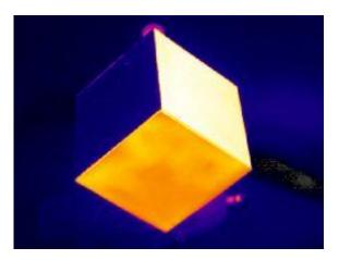
Figure 4. A Leslie cube. To demonstrate the effects of surface emissivity, each side of this cube was coated with a different material. Although each side appears different when viewed through a thermal camera, the internal temperature is the same. Image: Brandenburg Technical University.<sup>4</sup>
