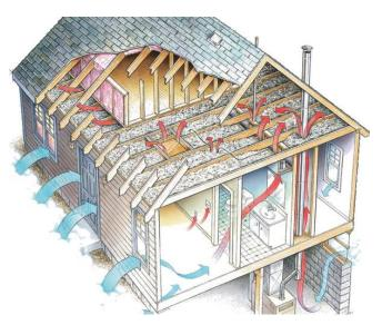
Figure 7. Warm air rises through a building, while cool convective air currents infiltrate through the gaps in the structure's air barrier. Image: All In One Insulation.<sup>7</sup>
