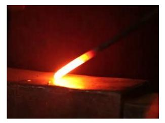
Figure 1. The hottest part of this iron rod glows with white light. Further from the tip, the light shifts from yellow, to red, and then to infrared (which is not visible). Image: Shutterstock<sup>1</sup>.
