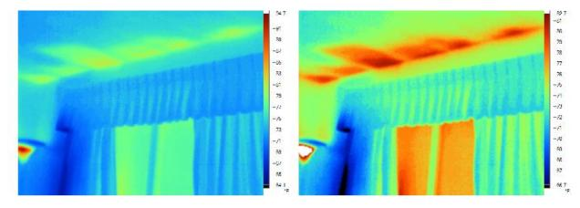
Figure 9. Two thermal images of a room with a light fixture and a large window. Although the scene is identical and the colour gradient is the same, the instrument's readings are displayed using different temperature spans. Image: Thermal Imaging Blog.<sup>9</sup>
