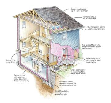
Figure 6. Cross section showing a building's outer shell and layers of thermal insulation. Image: Green Building Advisor.<sup>6</sup>
