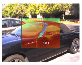
Figure 2. Infrared radiation reflected off a chrome strip. Image: MoistureView.<sup>2</sup>
