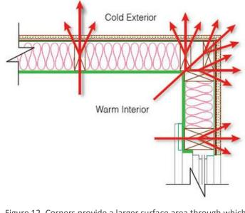
Figure 12. Corners provide a larger surface area through which heat can be transferred. Image: AIA/Architectural Record Continuing Education Program<sup>12</sup>
