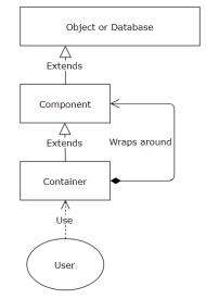
Figure 6 - Component Container Pattern
