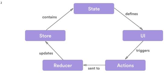
Figure 3 - Redux React Workflow
