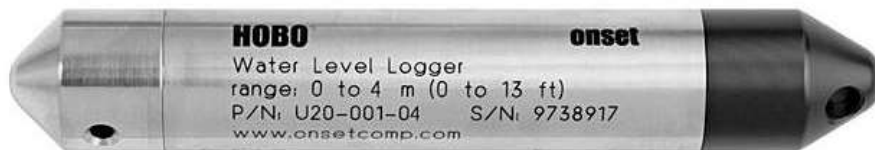
Figure 42: HOBOTONSET U20-001-04 pressure transducer
