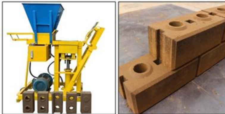
Figure 21: Stabilized Mud Blocks production technology 18
