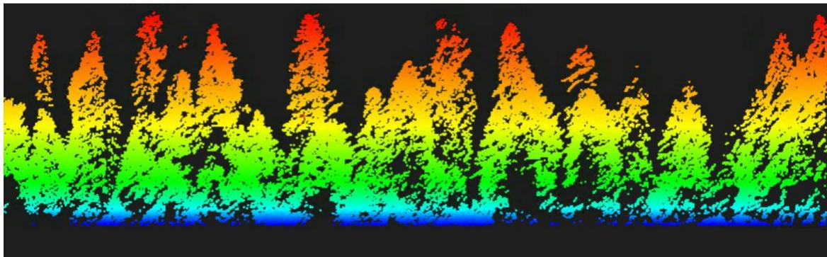
Clip of Lidar Data from Orchid Creek area. Maximum tree height is 70 m
