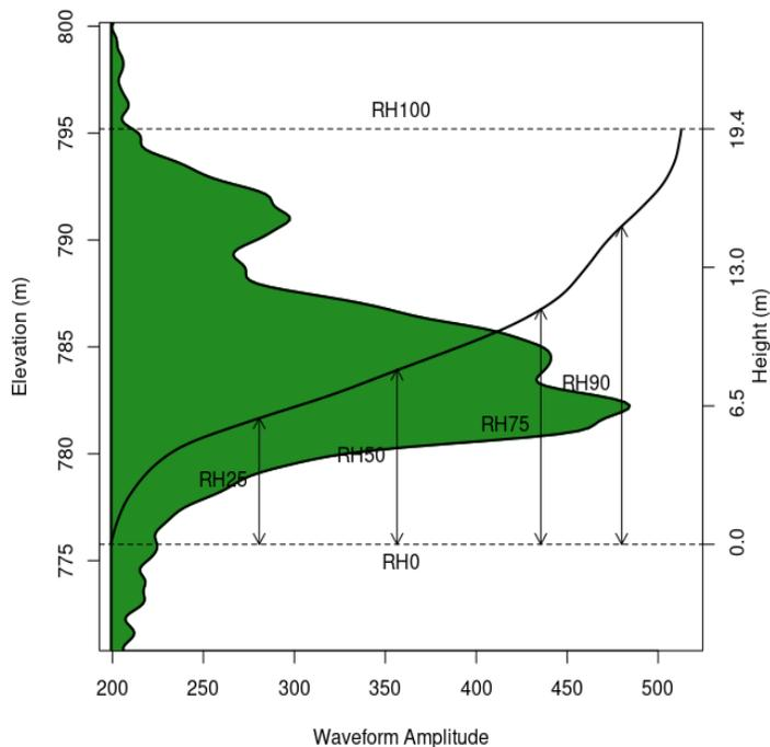
Figure 6. Example GEDI pulse waveform. Amplitude is the return strength, where most of the light is reflected. RH0 is considered ground, and RH100 is the top of the canopy. Image source: Sylvia et al., 2020.
