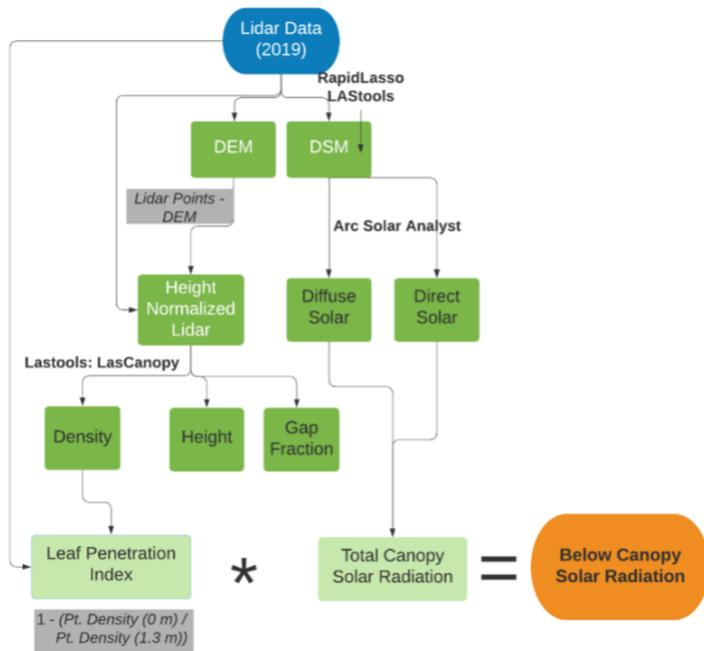
Figure 3B includes an overview of methodology for solar radiation estimates at cedar dominant sites. At these sites, Lidar point clouds were used to build a model of topography - digital elevation model (DEM), and canopy, including both a digital surface model (DSM) and a canopy height model. The lidar point cloud was normalized to topography to isolate lidar point returns associated with vegetation. Following normalization,
