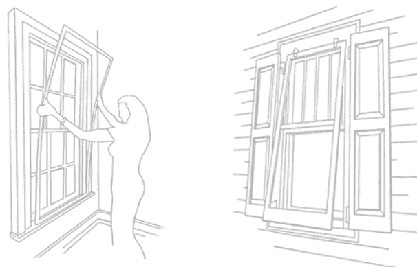
An image of exterior storm windows on the exterior of the original wood-framed window and the installation process. Source: vintagewoodworks and Indow Windows
