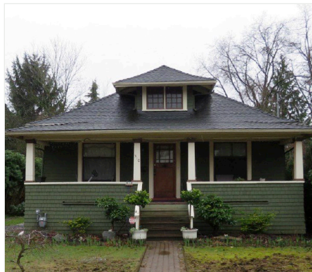
Porches were designed to cool off exterior walls, allow windows to be opened all year long and provide a sheltered living space.
