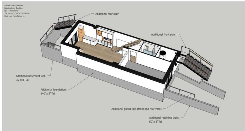
Figure 9 additional materials required for fulfilling basement requirements – credit: Lanefab
