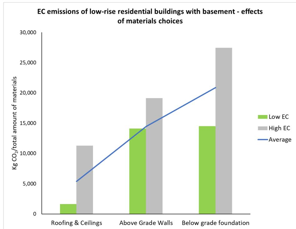
Figure 6 Effects of materials choices on the EC emissions of low-rise residential buildings with basement
