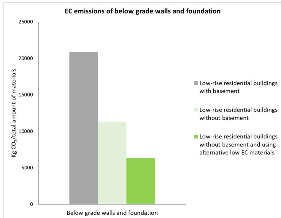
Figure 8 Effects of basement removal and application on alternative low EC materials on the EC emissions of below grade walls and foundation
