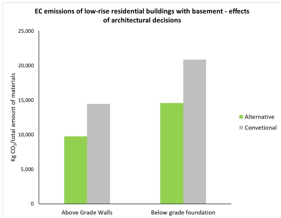
Figure 7 Effects of architectural decisions on the EC emissions of low-rise residential buildings with basement
