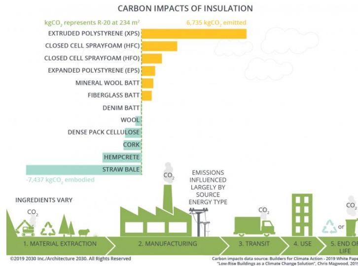
Figure 3 Carbon emissions (kg CO<sub>2</sub>) of different types of insulation (3)
