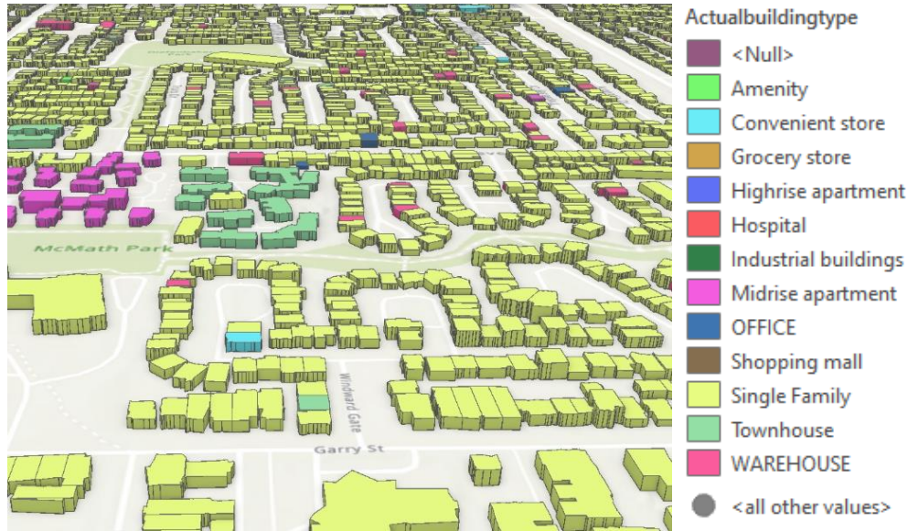
Figure 6 3D Richmond city building model after classifying LiDAR point cloud, yellow color for the archetype of single family, pink for industrial building, purple for low-rise apartment, green for townhouse.
