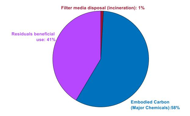
**Figure 1** Major identified areas of non-energy emissions at Coquitlam Water Treatment Plant (CWTP) and Seymour Capilano Filtration Plant (SCFP) and their estimated fractional contributions. *Note: Emissions from UV disinfection systems and refrigerants are not included in this breakdown due to limited data availability but are assumed to be minor compared to the sources above, based on process review*
