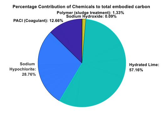
Figure 2 Relative CO₂e contribution of a few major treatment chemicals based on available data. Certain treatment chemicals (proprietary) are excluded from this chart due to limited carbon footprint information; the intent is to highlight the major contributors.
