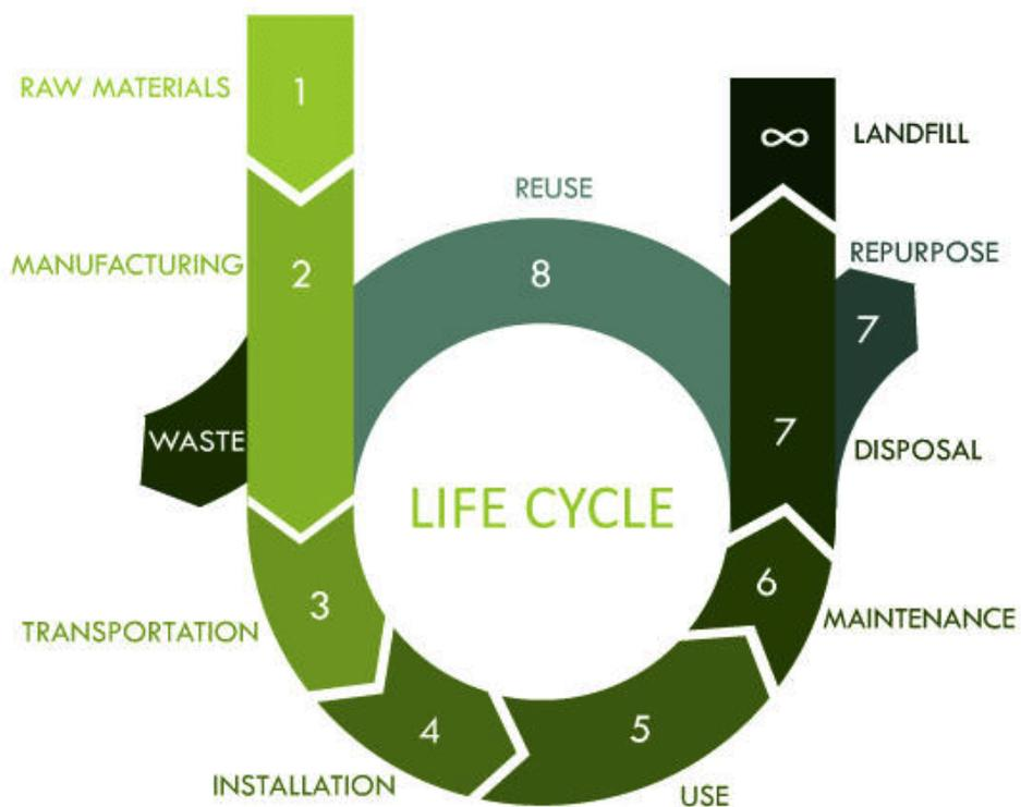
Figure 1: Flow diagram illustrating both cradle-to-grave and cradle-to-cradle product lifecycles (Source: Southwest 2016)
