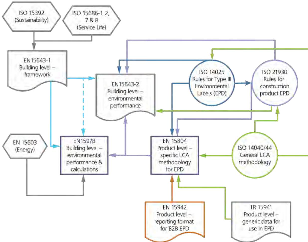
Figure 6: Interactions between environmental assessment EN and ISO standards (BRE 2016)
