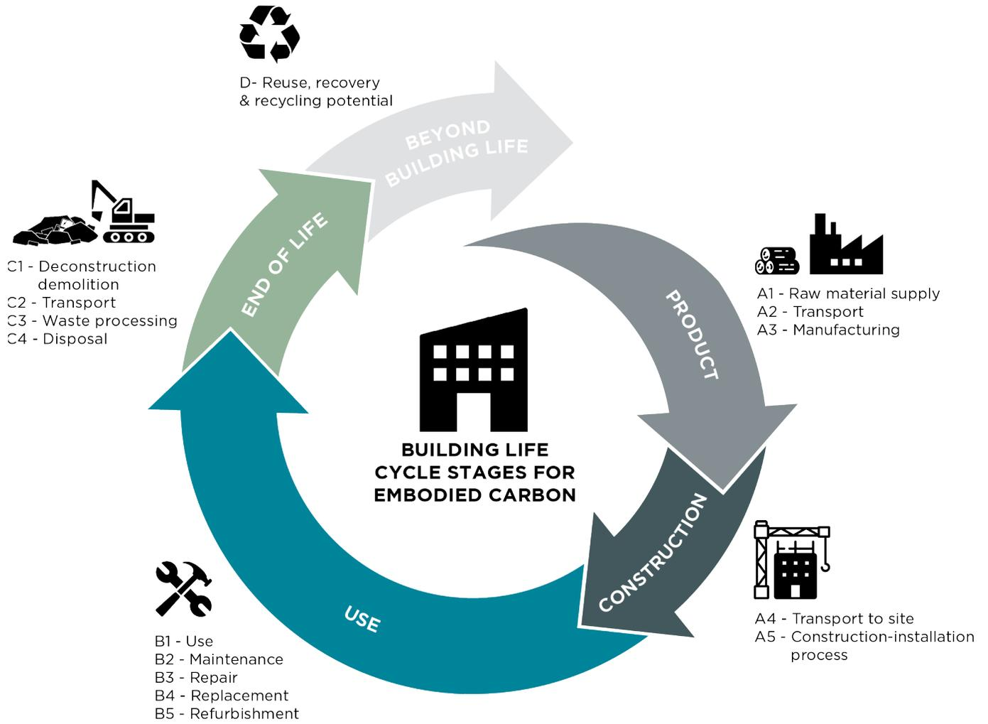
Figure 2: Embodied carbon building life cycle stages and modules per EN 15978:2011<sup>6</sup>
