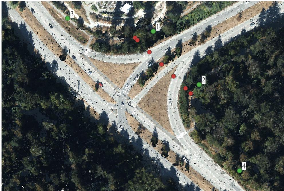
Figure 12: Overpass Ramp Extents (Green) Visualization on Site LiDAR
