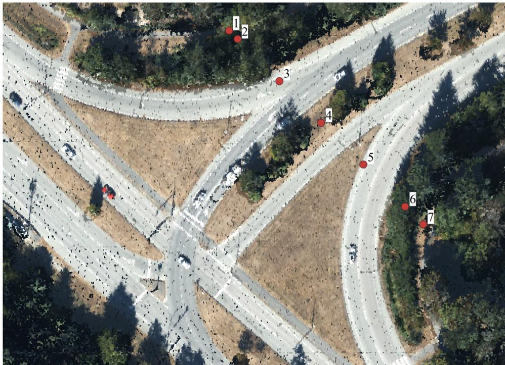
*Figure 11: Overpass Column Placement Visualization on Site LiDAR*
