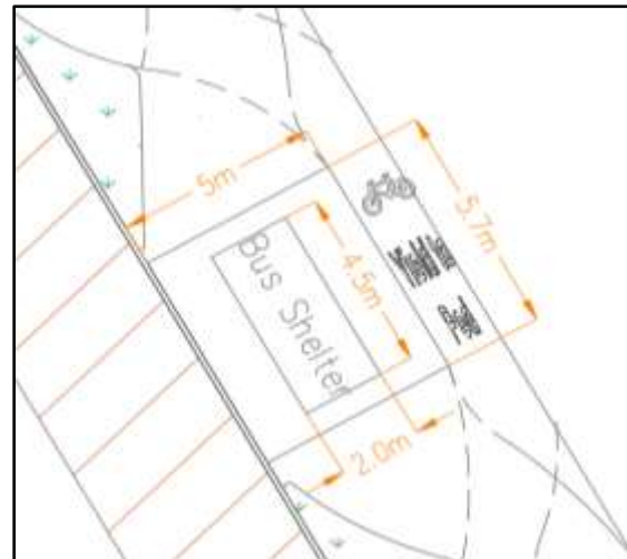
Figure 4 Bus Stop Configuration
