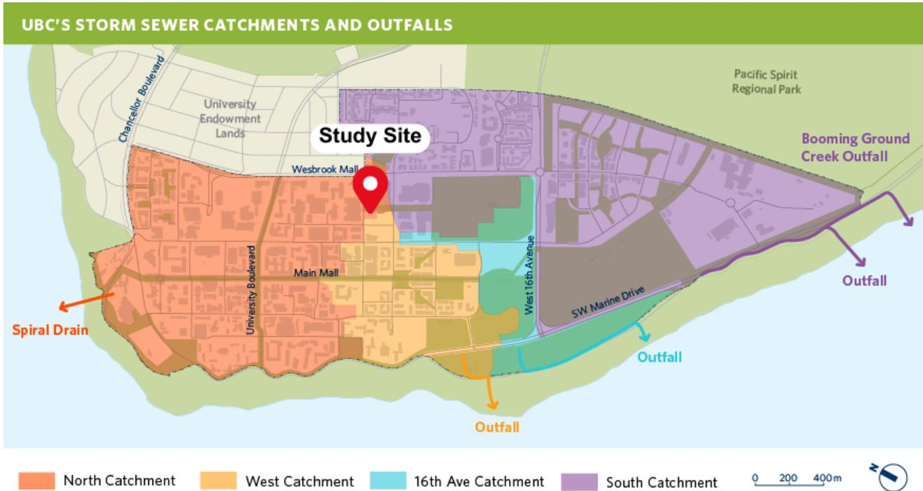
Figure 3. Map of UBC's Storm Sewer Catchments and Outfalls, with the study site indicated by a red marker (UBC Facilities: Energy & Water Services, 2017).
