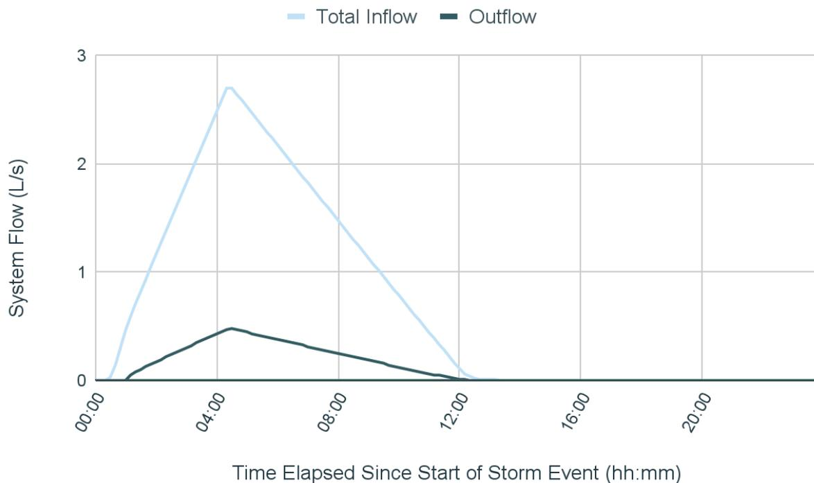
Figure 15. Comparison of total system inflow (L/s) and system outflow (L/s) over time elapsed since the start of the storm, for a storm event with a 10y return frequency and a 12h duration.
