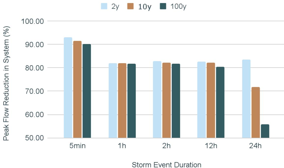
Figure 16. Peak Flow Reduction of the system (%) per each storm event. Storm events are characterized by storm duration by the frequency of the storm event. Storm frequency is given as 2-year events (light blue), 10-year events (brown), or 100-year events (dark green). Peak flow reduction was calculated using the peak total system inflow and the peak system outflow outputs generated in the SWMM model after running each storm event.
