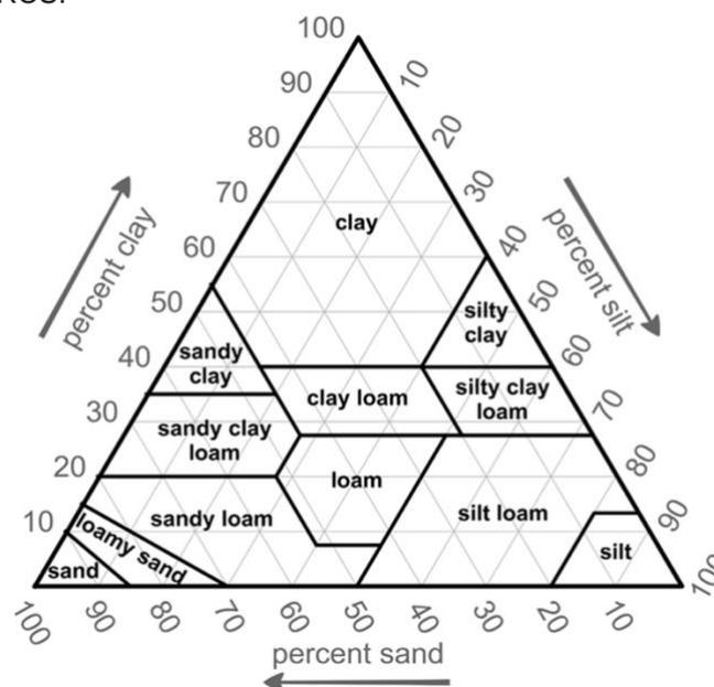
Since the SWMM software was developed in the US, US-based soil texture classification was used for the model. Input values for these parameters were outlined in Table A.2 Soil Characteristics of the US EPA SWMM 5.2 User Manual (Lewis A. Rossman & Simon, 2022).
