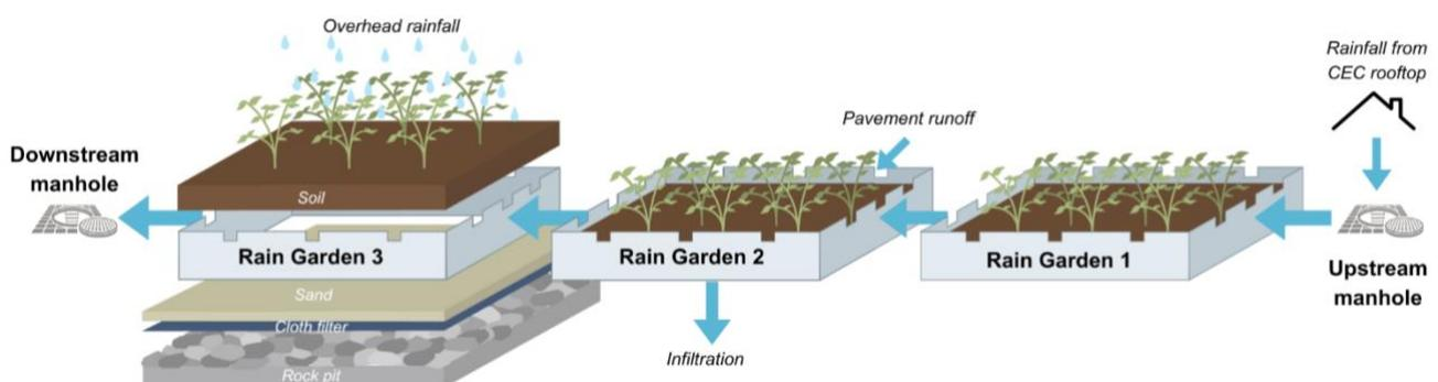
*Figure 1.* Simplified illustration of the study site's system of three RGs. Blue arrows represent the flow of water. After passing through the downstream manhole, water is then directed to a detention tank and drained into existing storm sewer infrastructure as part of the North Catchment, which eventually discharges into the ocean.
