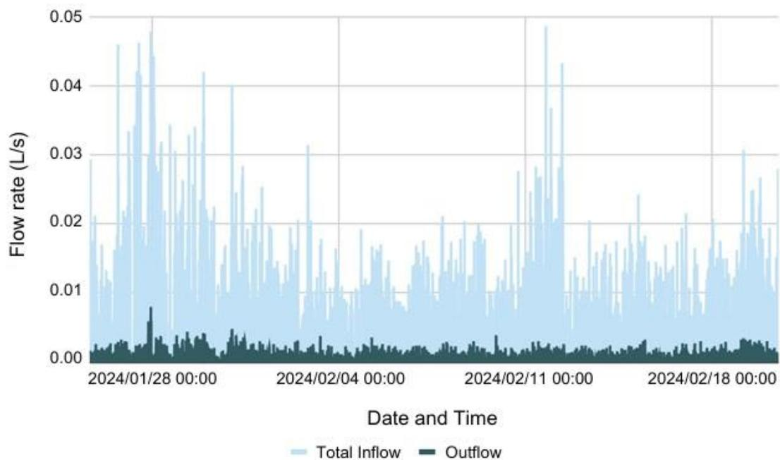
*Figure 12.* Total inflows and outflows (L/s) from the CEC RG system from January 25<sup>th</sup>, 2024 to February 20<sup>th</sup>, 2024. Measurements were taken in 5-minute intervals. Total inflow is the sum of the total precipitation inflow, the initial inflow, and the water flow into the RGs. Outflow was measured through a logger placed in the manhole downstream.
