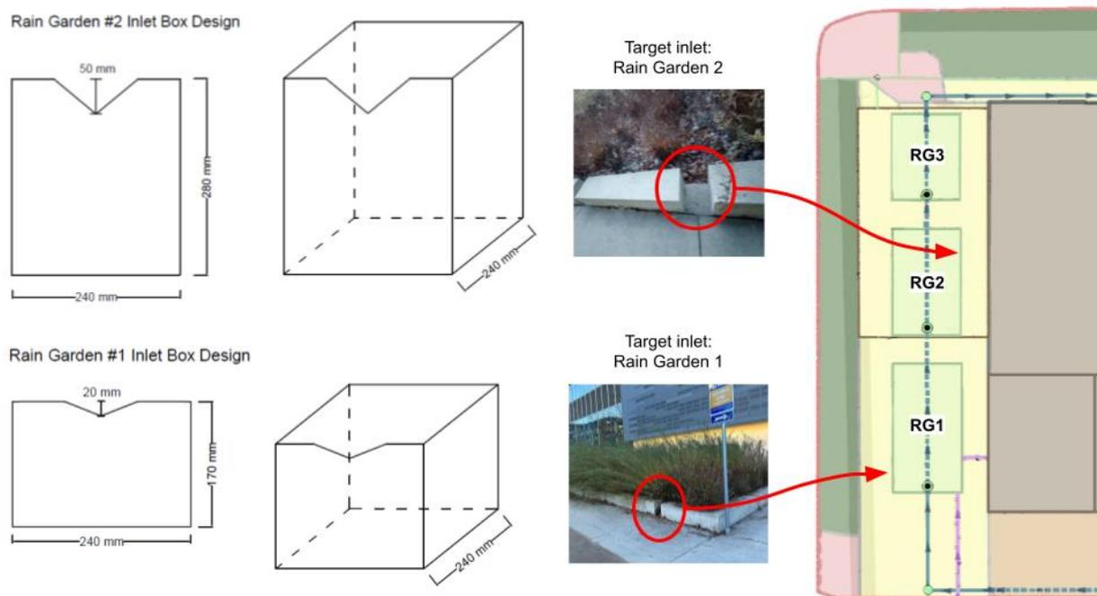
Figure 6. Weir box design with dimensions for both RG 1 & 2.
