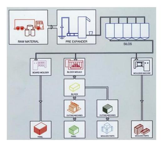
Figure 11: A typical production cycle in a Polystyrene plant <sup>[23]</sup>
