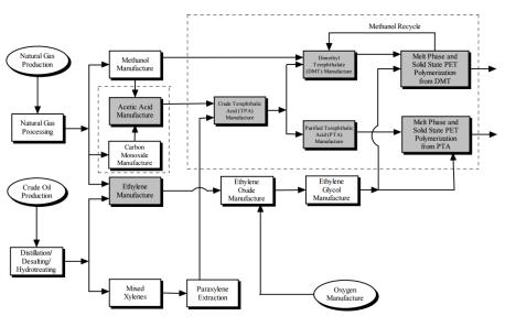
Figure 6-1. Flow diagram for the manufacture of virgin polyethylene terephthalate(PET) resin. Shaded boxes represent partial or complete data provided by manufacturers specifically for this analysis. Boxes within the dotted rectangle are included in an aggregated dataset.
