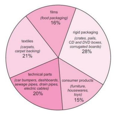
Figure 14: How polypropylene resin is used in manufacturing <sup>[34]</sup>.
