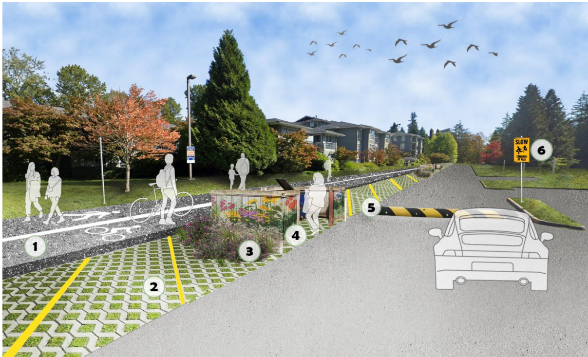
Figure 8: Perspective View 1 illustrates recommendations along the Melfa Rd: (1) Repurpose original perpendicular parking into 45°, expanded area can be used to widen sidewalk and introduce a separate bike lane; (2) use permeable pavement instead of hard pavement; (3) add rain gardens beside dumpsters to improve biodiversity; (4) add paintings on dumpster fences, which could be done by kids; (5) add a speed bump to better moderate vehicular speeds; and (6) add SLOW signages to warn drivers there are kids ahead.
