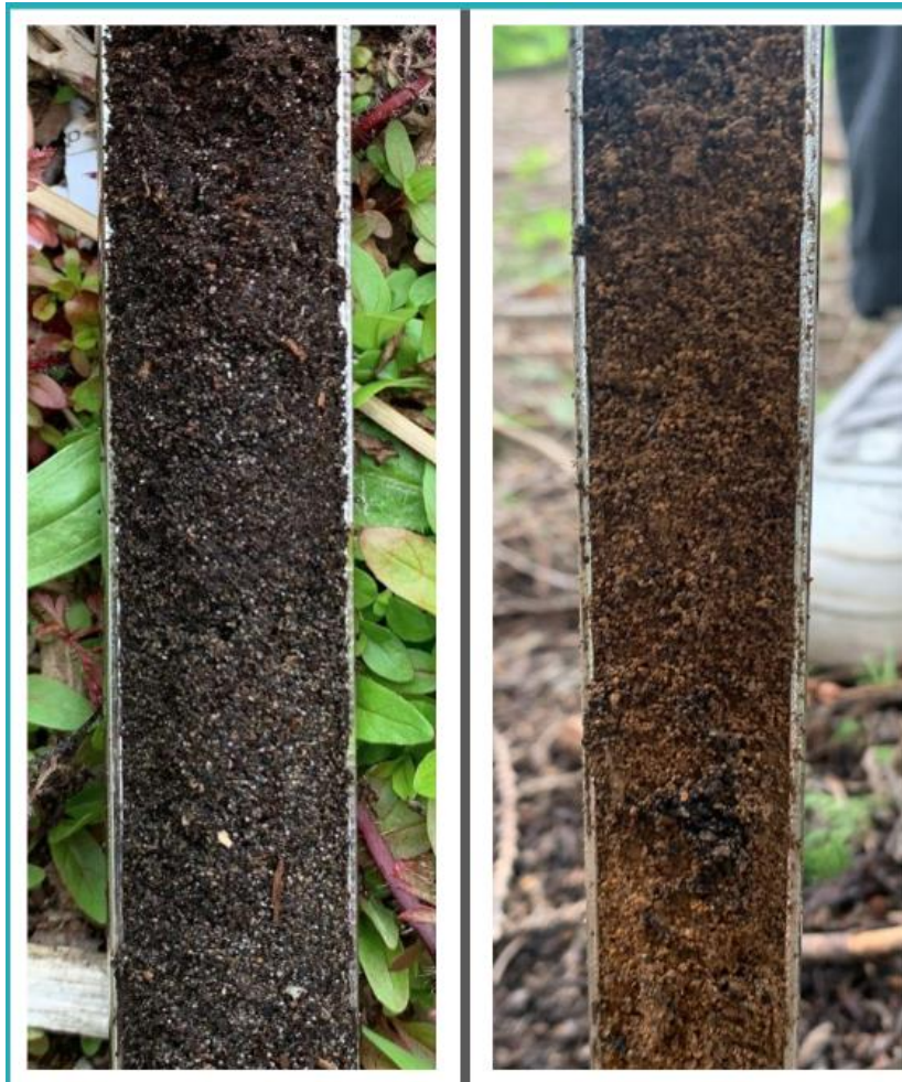
Figure 1 - The push tube sample on the left is a MSB while the sample on the right is native soil. One key feature of the MSB is the uniform white sand particles.
