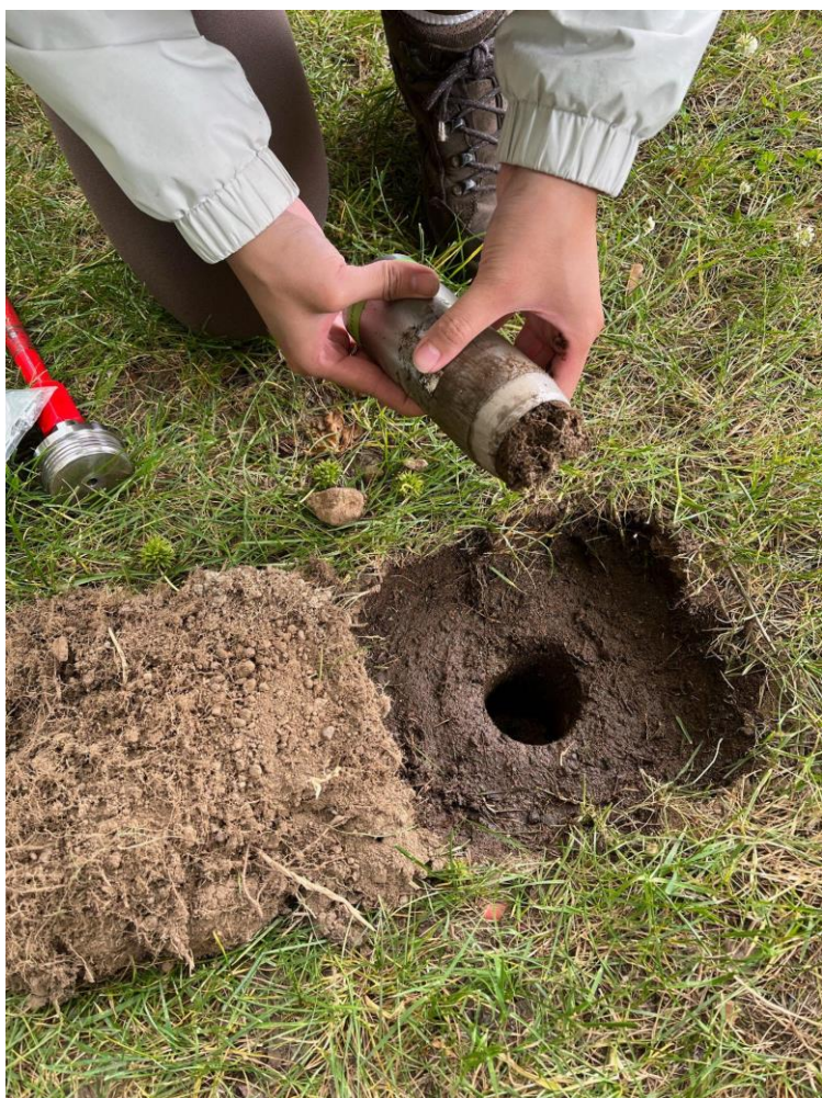
Appendix A - Photo of field data collection for bulk density cores. Each site was irrigated prior to using the bulk density hammer because the texture of MSBs were too sandy to collect dry core samples.
